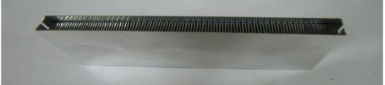
A view of the sandwich construction of the air side plain fins for the preliminary heat exchanger before dip brazing
